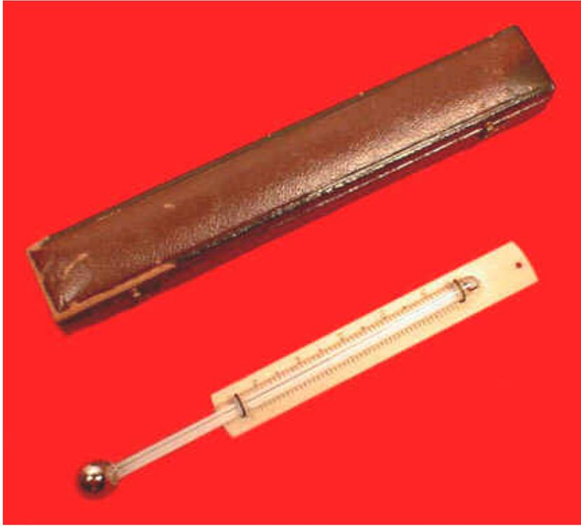
Figure 3. A pocket-sized medical thermometer circa 1850. This thermometer, with its ivory scale in degrees Fahrenheit, and its bulb projecting approximately one inch from the scale card, is likely very similar to the ones used by Dr. Davy on his 1816 voyage.
