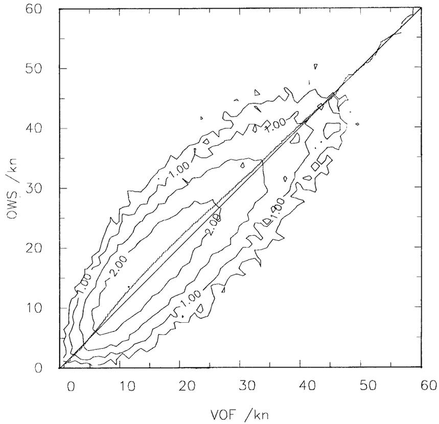
**Figure 8: New Beaufort equivalent scale based on reduced OWS measurements, therefore valid for a height of 10 m.**
